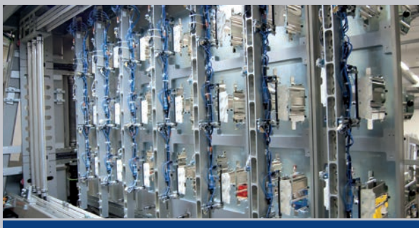
Label hand over from magazine to mandrel
