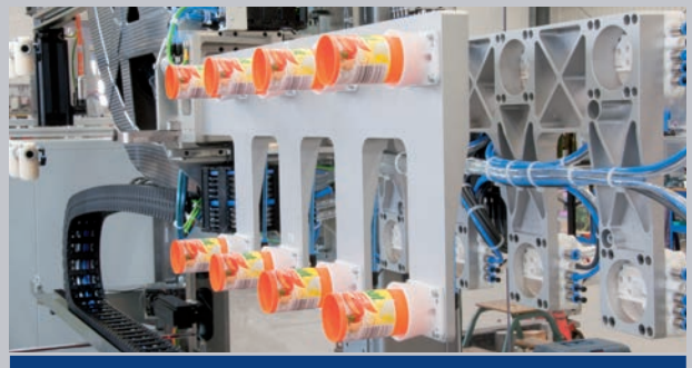
Carbon arm with AI-gripper for IML-system having 8 cavities
