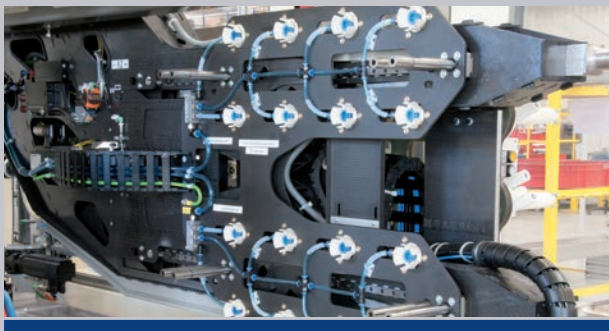
Carbon gripper for IML-system having 16 cavities
