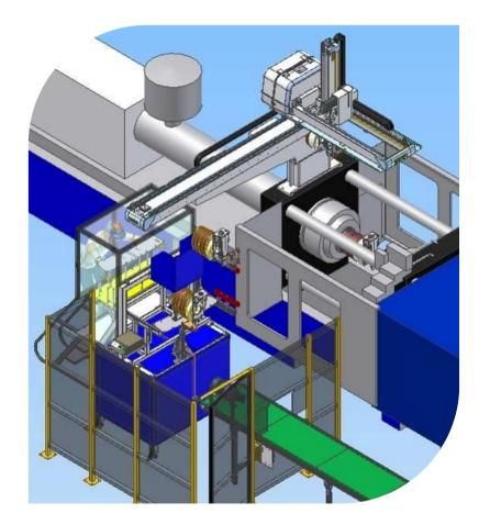
This is a really flexible solution for applications with cycle time >8 sec, used mainly for large size products. The open mould daylight is very little and standardised components are used as much as possible. The set-up time for production change is very short, so that the quantities of production is optimised.
